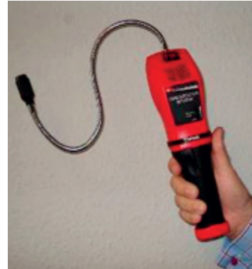
Figure 3 - Electronic leak detectors suitable for flammable refrigerants
